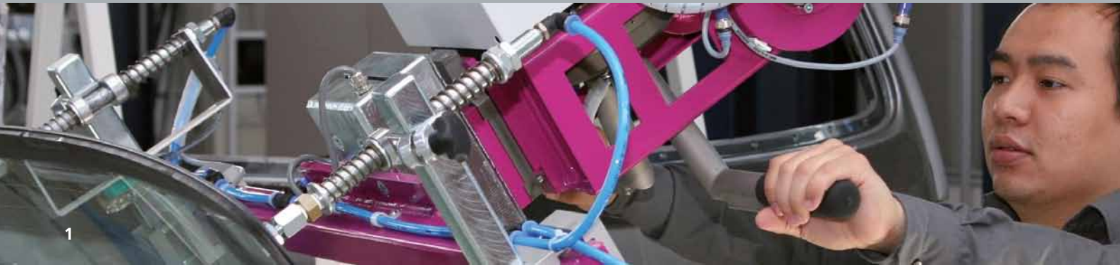
1 Partly automated screen assembly with cooperative robots
